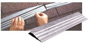
strip of copper or zinc coated sheet metal under the row of shingles near the ridge. Rain running over the metal creates a chemical reaction that will kill the algae. This is often visible at the chimney or under the furnace vents where they meet your roof. Additional information on installing zinc strips can be found at <a href="https://www.zincshield.com">www.zincshield.com</a> or <a href="https://www.z
